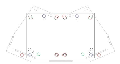
Single Horizontal Stasys X Attach feet to the 4 blue locations on the underside of the tilt board
