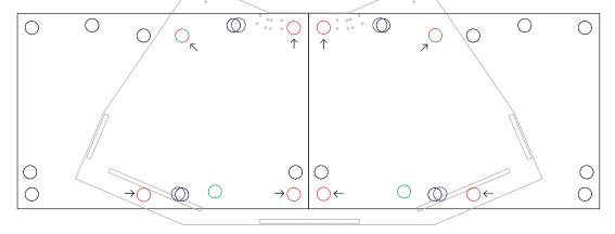
Dual Horizontal Stasys X Attach feet to the 8 red locations on the underside of the tilt board
